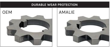
Gears from Inner Oil Pump: Noticeable wear on the gear using OEM fluid (left); no wear on gear protected by AMALIE Universal Synthetic ATF (right)
