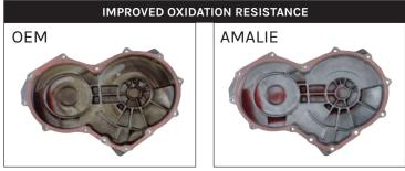
Transmission covers: OEM fluid (left) oxidized much faster (heavy deposits); AMALIE Universal Synthetic ATF (right) resisted oxidation (almost no deposits)
